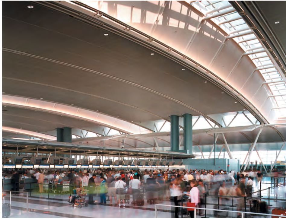
Cove lights along skylights and downlight
