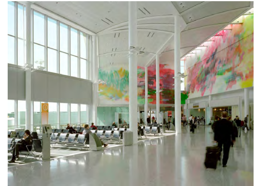
Uplighting integrated into structural columns
